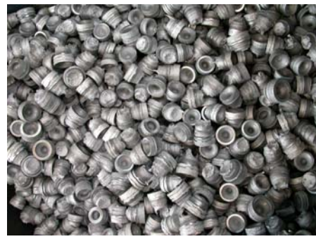
Punched out sprues for recycling
