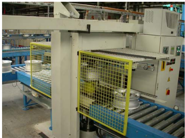
Continuous automatic desprue machine line
